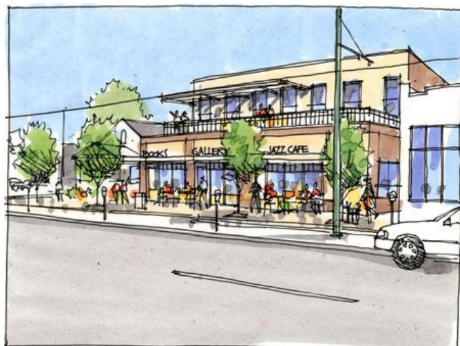
A sketch of how to add to an existing one story retail building.
